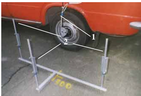
Fig. 4. Optical system (1 – optical sensors, 2 – reflectors on brackets)
