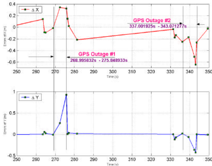
Fig.17. Errors of the longitudinal ( \Delta X ) and lateral ( \Delta Y ) coordinates in the absence of signals from both GPS and the optical system (the experiment “Movement at maximum speed”)
