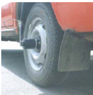
Fig. 6. Odometer fastening on a wheel
