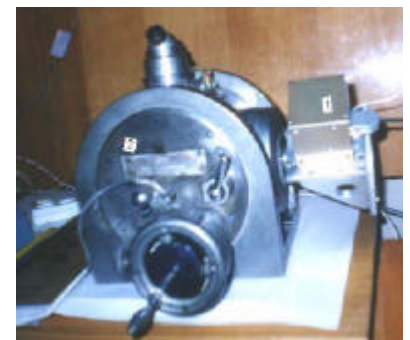
Fig. 9. The installation for the odometer and optical sensor calibration (1- a motor; 2 – the odometer; 3 – a disk with an optical reflector; 4 – an optical emitter and receiver)
